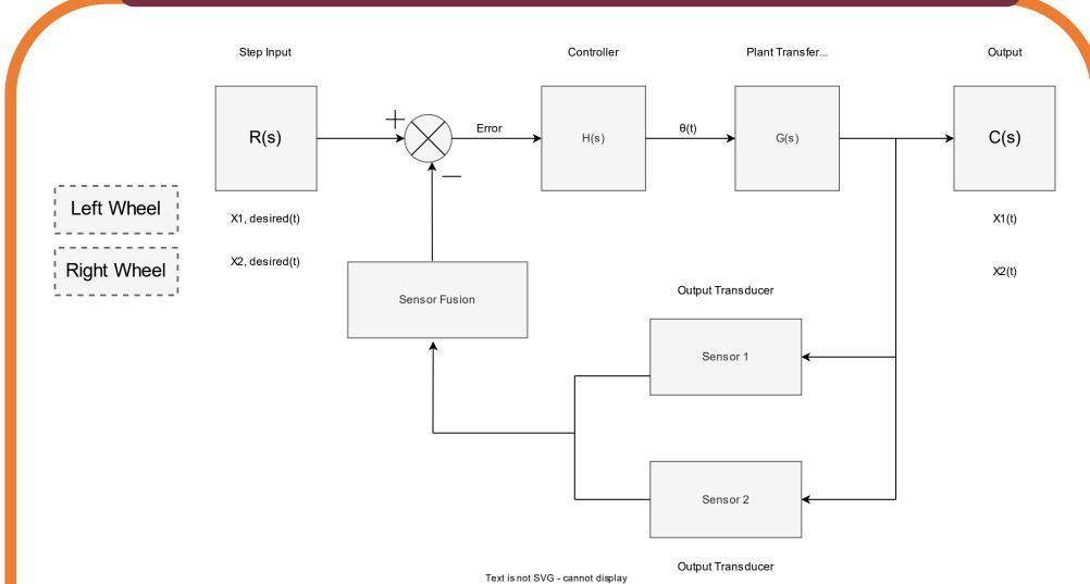
The step input is the desired position of the wheels along the cylinder. The transfer function is derived from inverse kinematics. Position is then sensed and consolidated. The controller applies a gain to the error based on the control input.
