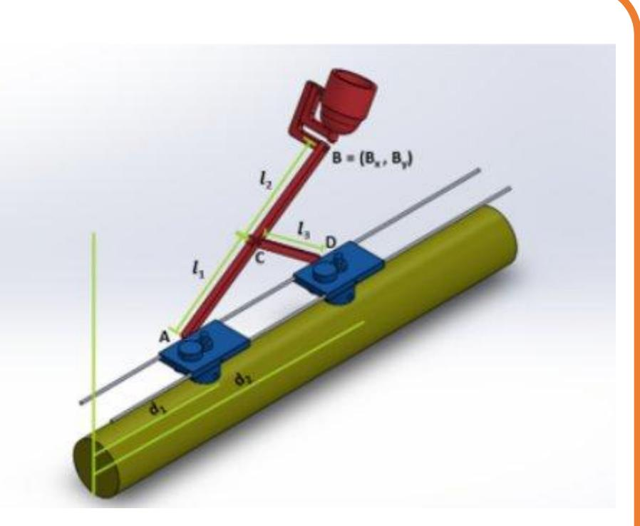
Wheels (blue) are steered on a cylinder (yellow), changing the system's effective gear ratio. The translational velocity of each wheel is changed, moving a point (red) in two-dimensional space.
